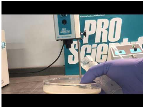
Seeds, pulp and pumpkin chunks homogenized with the SB-1, PRO250 and Multi-Prep Homogenizers
